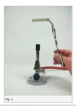
Remove the polyethylene sample from the flame, hold it for a while over the work-plate. Proceed in the same way with other plastic samples: polypropylene, polystyrene, cellulose acetate, polyurethane, silicone rubber.
