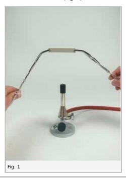
Remove the polystyrene piece from the burner flame and continue holding it over the work-plate. Proceed in the same way with polymethylmethacrylates and phenolic resin.
