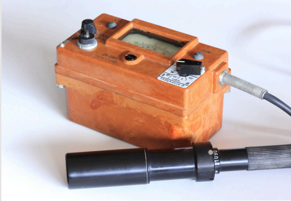
Geiger-Müller detector with visual display and acoustic signal
