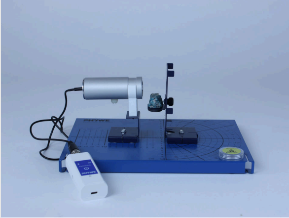
Test setup without absorber material in the beam path
