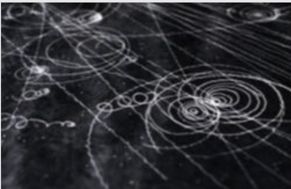
Different types of radiation in the magnetic field, made visible by a cloud chamber
