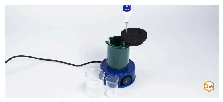
Students learn to experimentally record and quantitatively evaluate the heat absorption of an endothermic neutralisation reaction.
