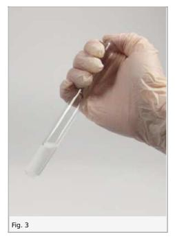
Pour into a second test tube the same quantity of mixture of Fehling's solutions I and II and heat the contents of both test tubes to boiling.
