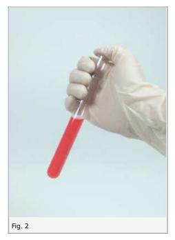
Into the faintly pink-coloured mixture place 20 drops of olive oil. Close the test tube again with your thumb, carefully turn the tube upside down a few times and put it in a test tube rack. In a few minutes the oil settles at the top of the tube.
