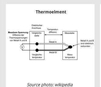
Thermocouples are used to measure temperature and generally consist of two different metals (or semiconductors) that are electrically connected at one point.
