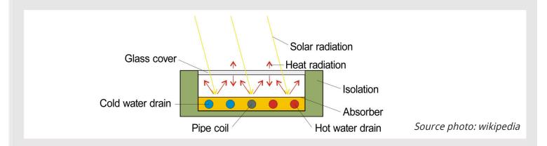
The incident solar radiation is converted into thermal energy by absorption and transferred to a liquid flowing through it.
