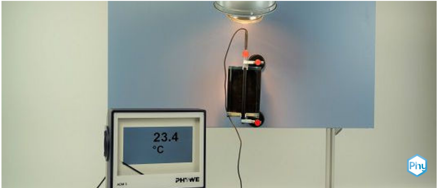
Heating water with a parabolic trough
