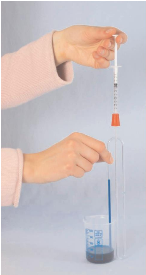
Fig. 2 Bubble-free filling of the U-tube
