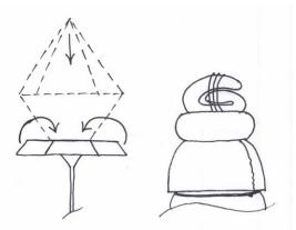
Once the parachute has been folded, wrap the ribbon loosely around the resulting parcel. Place the parachute with the polystyrene ring on the rocket dome. The sanded side of the polystyrene ring lies on the dome of the rocket.
