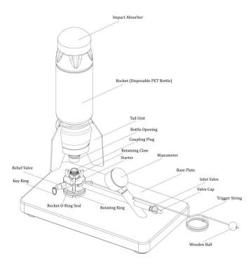
With this experimental set-up, the principles of a rocket (impulse, actio = reactio) and pneumatics can be covered and quantitative evaluations can be made depending on pressure, water quantity, aerodynamic design and weight (impact absorber).
