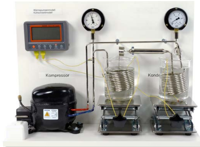
Fig. 1: Heat pump, compression principle 04373-93 (P2360202)
