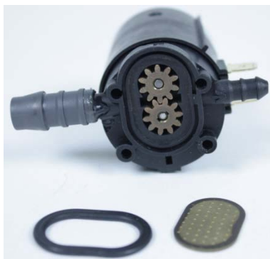
Fig. 4: Cleaning of the cog wheels inside of the pump.
