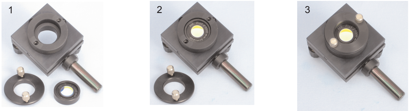
Fig. 9: Assembling the resonator mirror.
