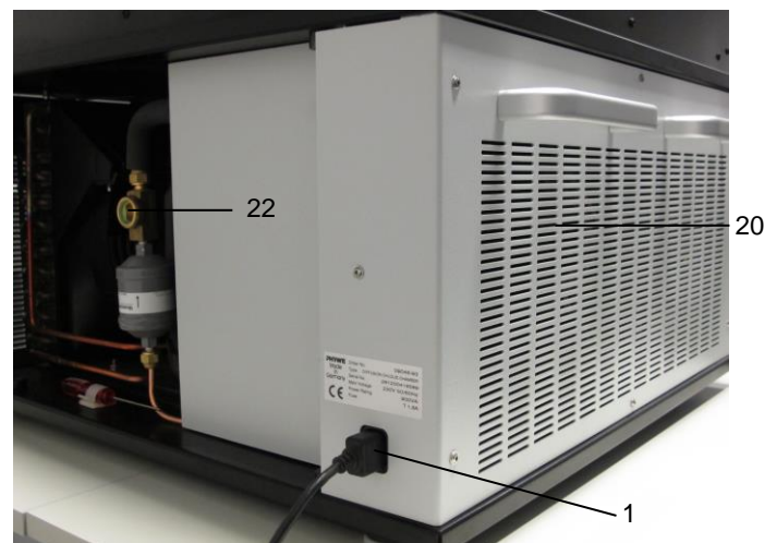
Fig. 5: Opened rear panel with cooling unit
