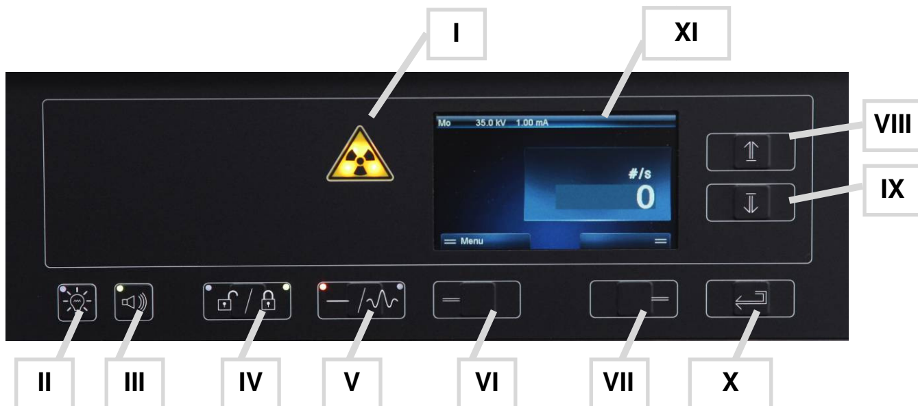
Fig. 3: Control panel at the front of the unit
