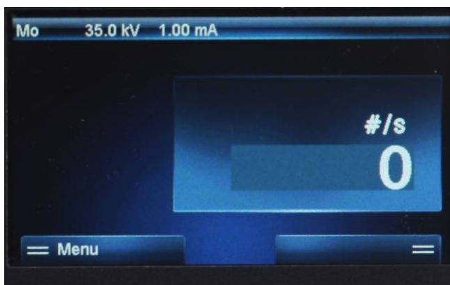
Fig. 7: Screen for controlling the unit at the front of the unit. The x-radiation is not activated.
