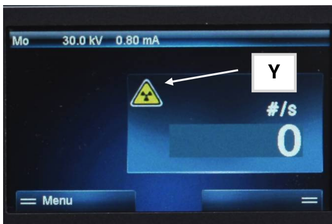
Fig. 7: Screen for controlling the unit at the front of the unit. The x-radiation is not activated.
