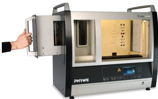
Fig. 4: X-ray plug-in unit on the left-hand side of the unit
