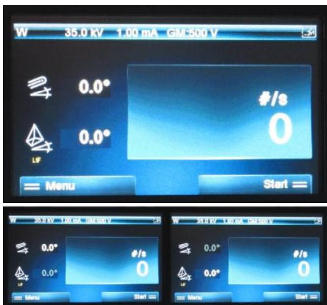
Fig. 4: top: coupled mode, left: rotate detector, right: rotate crystal.
