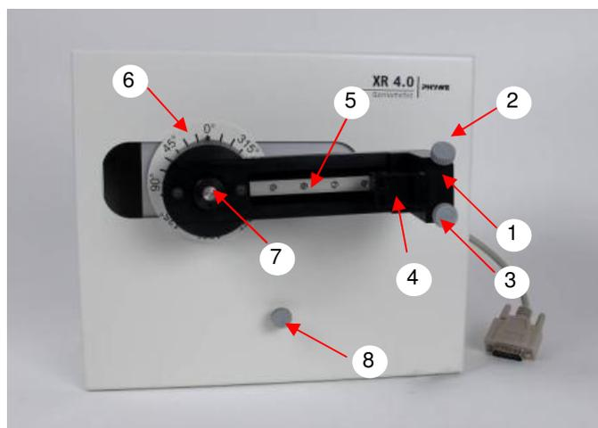
Fig. 2: Front view of the goniometer
