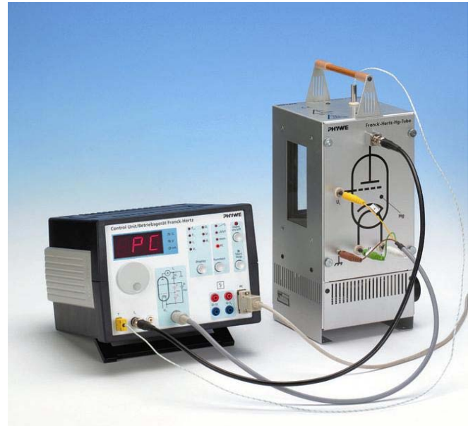
Fig. 2: Franck-Hertz experiment with Hg-Tube and oven
