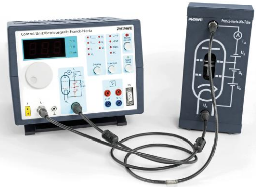
Fig. 3: Experimental set up of the Franck-Hertz experiment with Neon tube
