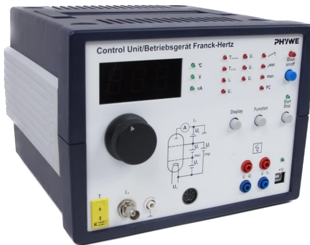
Fig. 1: Franck-Hertz Control Unit, USB 09106-99
