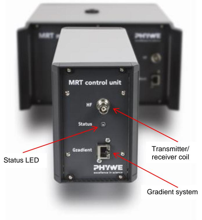
Fig. 2: Front of the control unit
