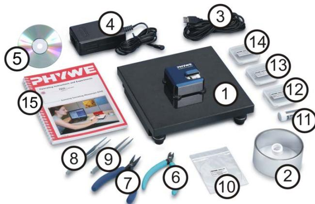
Fig. 1-1 Components of the PHYWE Compact STM.
