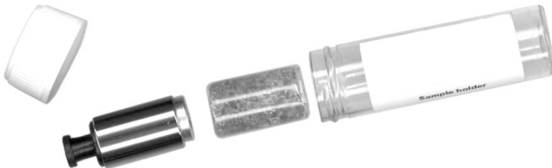
**Fig. 8-1 Sample holder and its package and silica container to prevent corrosion.**
