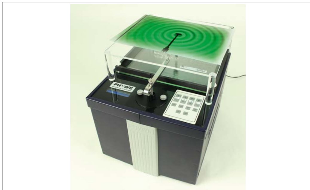
Fig. 1: Ripple tank with LED light source, complete 11260-88
