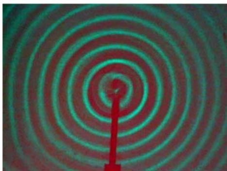
Fig. 7: Circular waves generated by the plug-shaped exciter.
