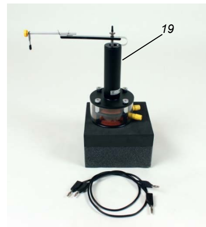
Fig. 6: External vibration generator (11260-10) with accessories, separately available.
