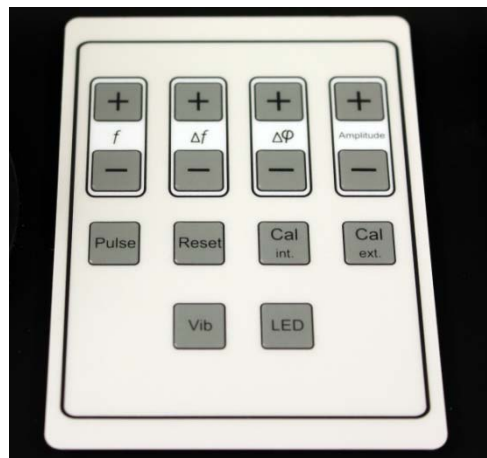
Fig. 3: The 14 keys control panel is situated on the top of the housing of the ripple tank.
