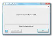
Connect the GAMMA-SCOUT® to the computer using the USB cable supplied. The data transfer process begins automatically and progress is indicated by a bar.
