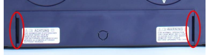
Fig. 5: Slots for removing the cover
