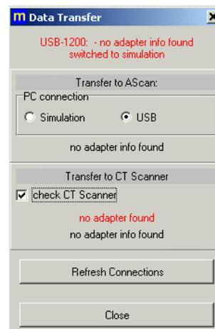
**measure Ultra Echo** Software can control the echoscope (13921.95) and the CT scanner control unit through an USB port or works in simulation mode. The respective setup can be entered in the "Data Transfer" window. To access select in the menu **Options** the item **Data Transfer**.
