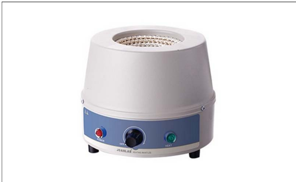
Fig. 1: Heating mantle for roundbottom
