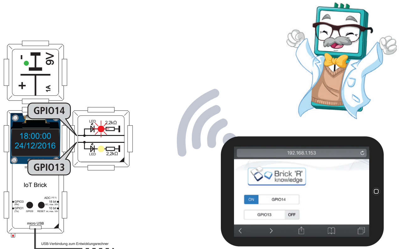
Fig. 13: Brick circuit "Switching via website"
