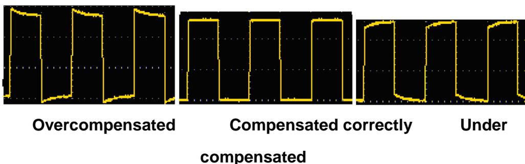
Overcompensated      Compensated correctly      Under compensated
