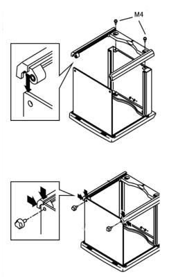
Push the side panels from the rear to the front into the guide frame. Make sure that the bore holes point towards the front plate.
