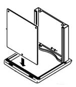
Make sure that the fastening point is placed at the frame in the bore hole of the front plate.
