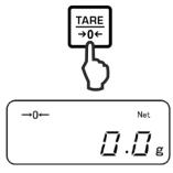
Wait for stability display, then press the **TARE** button The zero display and "**Net**" will appear.
