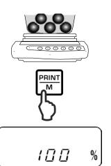
Place the reference weight (= 100 %) and confirm by pressing the **PRINT**-key.
