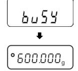
After successful adjustment the balance automatically returns to weighing mode.
