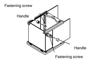
⇒ Fix the guide frame with two screws (M4).
