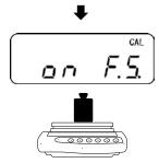
With display "on FS" place the required adjustment weight carefully in the center of the weighing pan.
