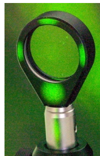
Figure 88 The first diffraction order does not fall on the lens.
