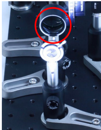
Figure 45: The aperture iris' shadow is centered on the condenser lens and its holder.
