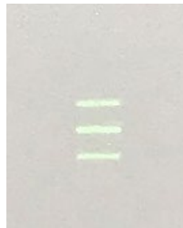
Figure 92: Diffraction Pattern in the Fourier Plane, Photographed on the Screen
