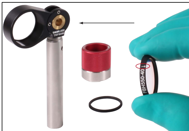
Figure 22: Assembly of the green filter: note the orientation indicated by the white arrow on the filter's mount.
