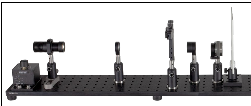
Figure 60: The Condenser Lens and the Objective Lens Form a Keplerian Telescope With a Magnification of 3/5
