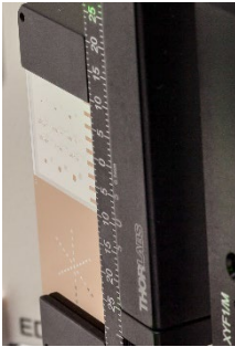
Figure 81: Babinet's Principle Demonstrated with Complementary Gratings
