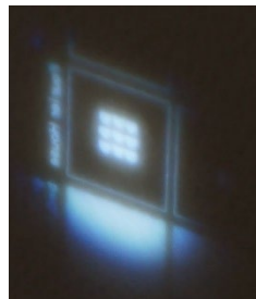
Figure 59: Photo of the Image on the Screen Created by the Keplerian Telescope Formed by the Condenser Lens and the Objective Lens
